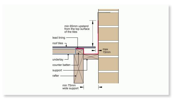
For pitches greater than 45° in sheltered and moderate exposure zones only. For pitches below 30°, evidence shall be provided as to suitable performance.
