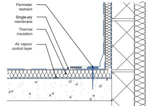
Warm roof systems with polymeric single ply membranes
