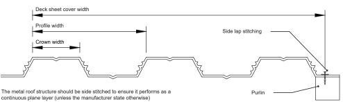
Profiled metal decks should conform to the following standards:
