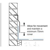
Where a timber frame structure abuts a masonry structure allowance should be made to accommodate movement in the timber frame and ensure the appropriate cover is maintained
