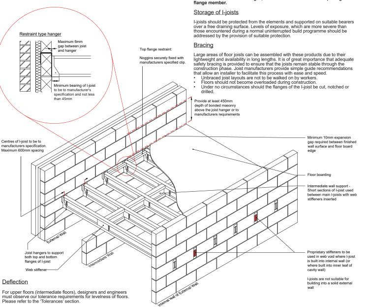
There may be an instance where a joist might be designed to meet permissible deflections within a relevant British Standard; however, our tolerance requirements will take precedence. The top and bottom flanges <u>must not</u> be notched. Where ceiling and floor boards are nailed to the flanges, care must be taken to avoid splitting of the
