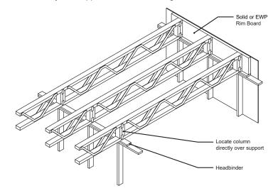
Example of metal web joists bearing on intermediate load bearing wall. Column within the metal web joist should be located directly over the support. In accordance with the manufacturers design
