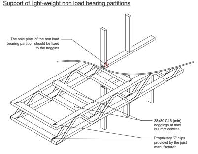
Where light weight non load bearing partition are parallel to the joists, they should be suitably supported in accordance with the manufacturers design.
