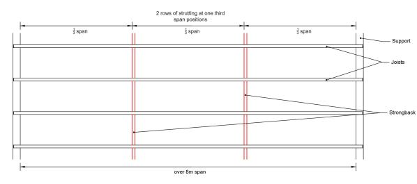
A minimum of two rows of strutting are required for spans over 8m. This should be provided by strongbacks in accordance with the manufacturers design.
