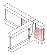
Fixing of multiple I-joists
