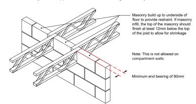
Metal web joists supported on load bearing masonry internal wall
