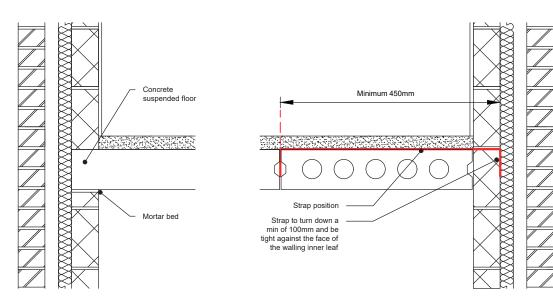
The floor units should bear onto masonry with a minimum 90mm bearing, and steelwork at a minimum 70mm
