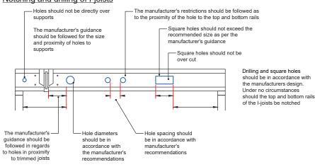
Trimmed openings may be needed around staircase openings and chimneys. Solid trimmed joists may be supported using joist hangers. Timber trimmers around openings should consist of at least two members and be designed and installed in accordance with the manufacturers instructions. Where an I-joist is faced fixed to another I-joists backer blocks should be provided on both sides of the web of the trimmer.
