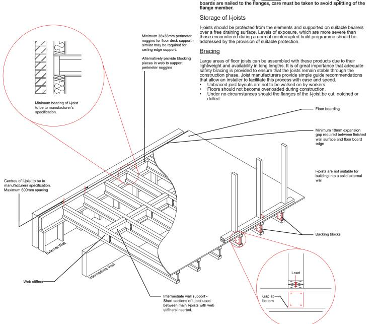
The top and bottom flanges must not be notched. Where ceiling and floor
