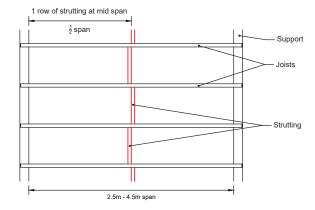
Where the span of a floor joist or flat roof joist is more than 2.5m, strutting is necessary. This should be provided either by timber bridging or strutting in accordance with the manufacturers design.
