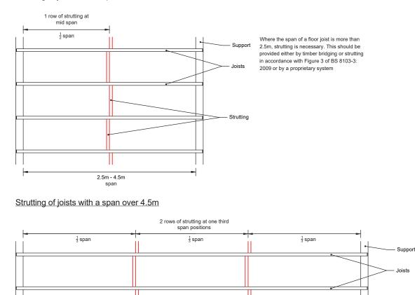
Nhere the span of a floor joist or flat roof joist is more than 4.5m, two rows of strutting at 1/3rd the span position will be necessary
