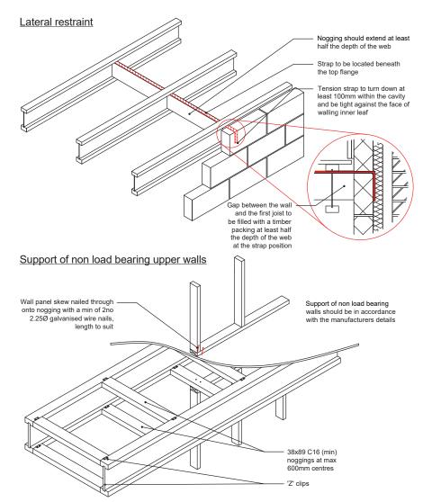
Straps need not be provided to floors at, or about, the same level on each side of a supported wall and at the following locations.
