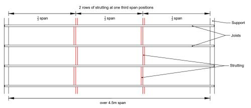
Where the span of a floor joist or flat roof joist is more than 4.5m, two rows of strutting at 1/3rd the span position will be necessary.
