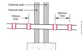
Where pipes are built-in, a connection on both sides of the wall to pipes with flexible joints located no more than 150mm from the face of the wall.
