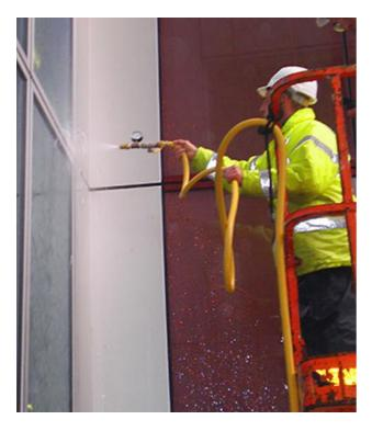
Hose pipe test attempts to replicate a negative internal pressure by spraying water at pressure. It is suitable for fixed joints only (sealed permanent joints). This test is not suitable for opening vents (windows/doors, as gaskets are too soft).
