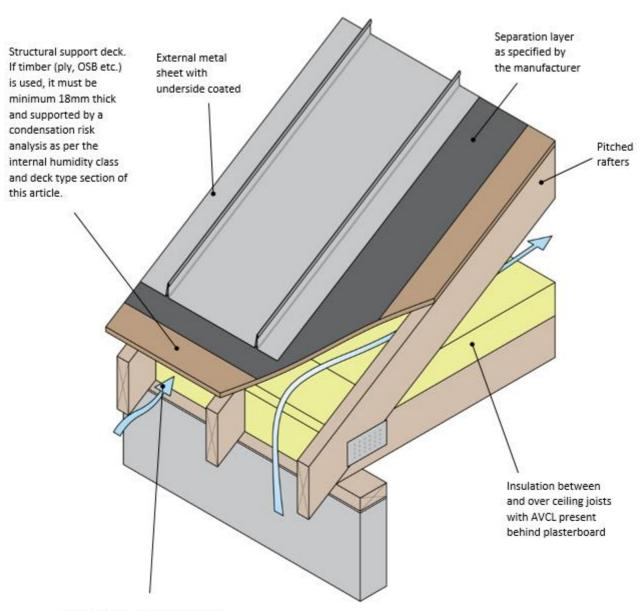
Eaves level ventilation to cold roof space to be provided in line with chapter 11 of our technical manual. Must be accompanied with high level ventilation at ridge level.
