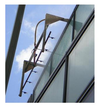
Spray bar testing is suitable for opening joints in curtain walling and sealed interfaces prior to rainscreen cladding being installed.
