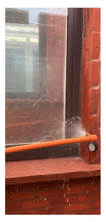
Pictured – Example of hose testing completed to panelised system in factory prior to required on-site testing.
