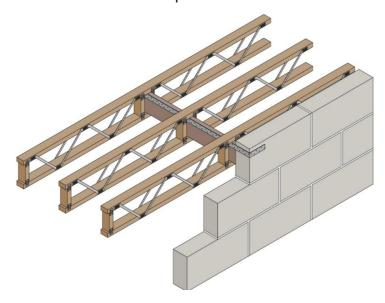
Restraint should also be provided for walls running perpendicular to joists by restraint type joist hangers.
