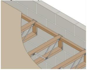
**8 -** Where studs above run parallel to joists, they should be supported on multiple joists or a row of noggins. Where they are supported on noggings, the soleplate for the stud should be fixed into the noggin. Where you see multiple fixings through the decking in a row, it may be due to a stud above not being supported or fixed into the noggins.
