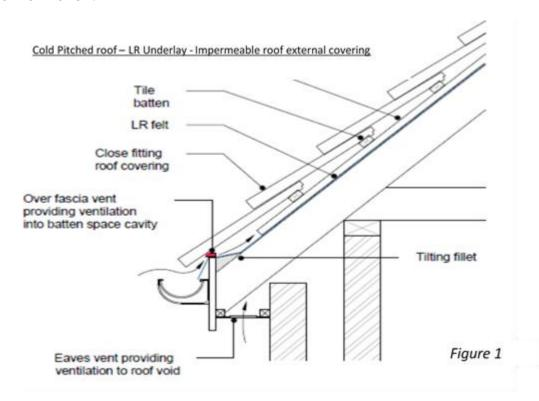
If the batten space is not ventilated, there needs to be an increased level of ventilation to the roof space and that should be in accordance with BS5250. The underlay manufacturer's 3rd party accreditation also needs to be followed. It is very difficult to determine a HR or LR underlay by sight alone and the manufacturer's third party accreditation should be referred to.
