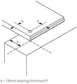
b = 8mm fixing distance (minimum)\* \*Dimensions taken from face dimension of board
