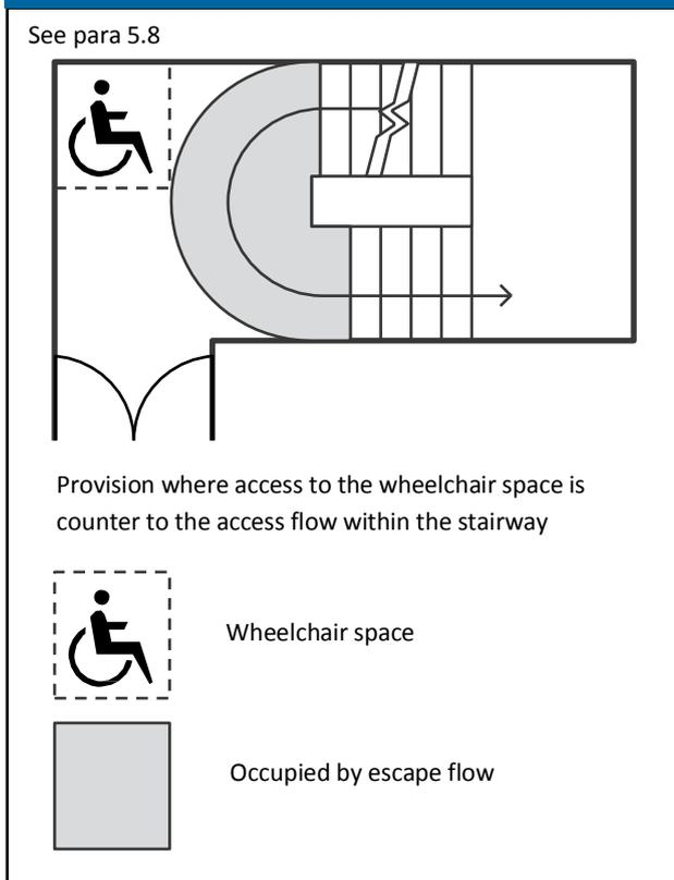
**5.10** Refuges and evacuation lifts should be clearly identified by appropriate fire safety signs. Where a refuge is in a lobby or stairway the sign should be accompanied by a blue mandatory sign worded “Refuge – keep clear”.
