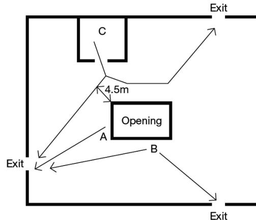
From A and B at least one direction of travel is away from the opening. From C where the initial direction of travel is towards the opening, one of the escape routes is not less than 4.5m from the opening.
