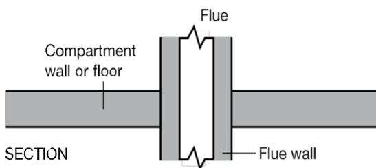
Flue walls should have a fire resistance of at least one half of that required for the compartment wall or floor, and be of non-combustible construction.
