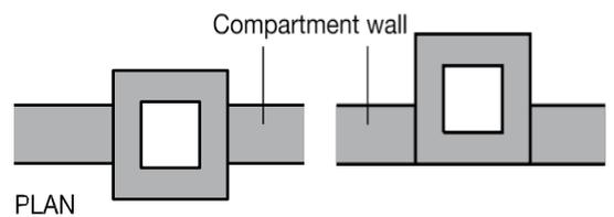
In each case flue walls should have a fire resistance at least one half of that required for the compartment wall and be of non-combustible construction.
