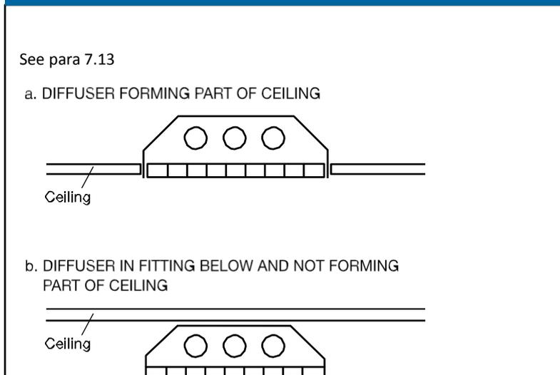
**7.14** Thermoplastic lighting diffusers should not be used in fire-protecting or fire-resisting ceilings, unless they have been satisfactorily tested as part of the ceiling system that is to be used to provide the appropriate fire protection.
