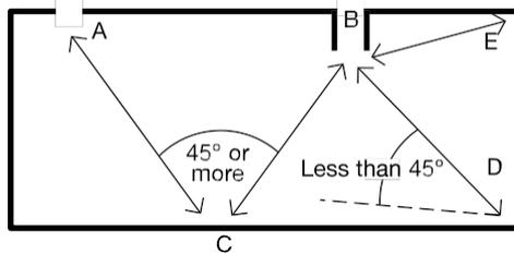
Alternative routes are available from C because angle ACB is  $45^\circ$  or more and therefore CA or CB (whichever is the less) should be no more than the maximum distance for travel given for alternative routes.
