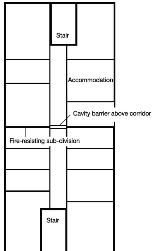
The sub-division should be carried full storey height and includes sub-division of the corridor. A cavity barrier may be used in any ceiling void over the sub-division.
