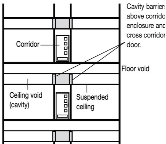
Where the corridor is a protected escape route, cavity barriers may also be required in any floor void beneath the corridor enclosure (see paragraph 10.4)
