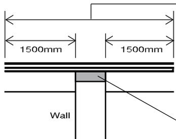
Roof covering over this distance to be designated AA, AB or AC on deck of material of limited combustibility. Roof covering and deck could be composite structure. E.g. profiled steel cladding.
