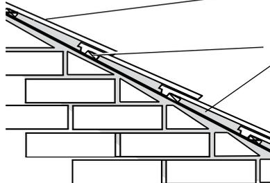
Roof covering to be designated AA, AB or AC for at least 1500mm either side of wall.
