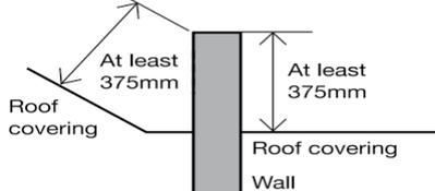
The wall should be extended up through the roof for a height of at least 375mm above the top surface of the adjoining roof covering.
