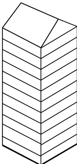
In a building over 30m in height all storeys should be separated by compartment floors. For advice on the special conditions in atrium buildings see BS 5588-7
