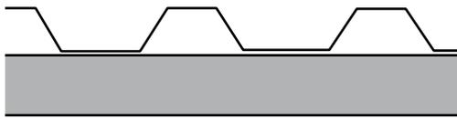
The insulation should make contact with both skins of sheeting. See also Diagram 30a regarding the need for a fire break where such roofs pass over the top of a compartment wall.
