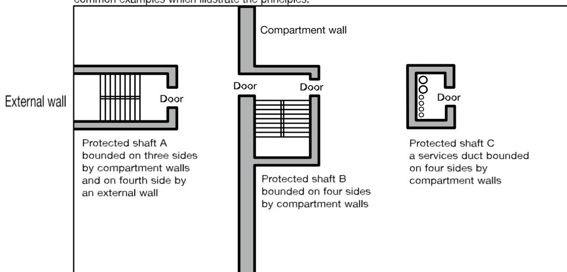
The shaft structure (including any openings) should meet the relevant provisions for: compartment walls (see paragraphs 9.20 to 9.34), external walls (see Sections 13 and 14 and Diagram 24)
