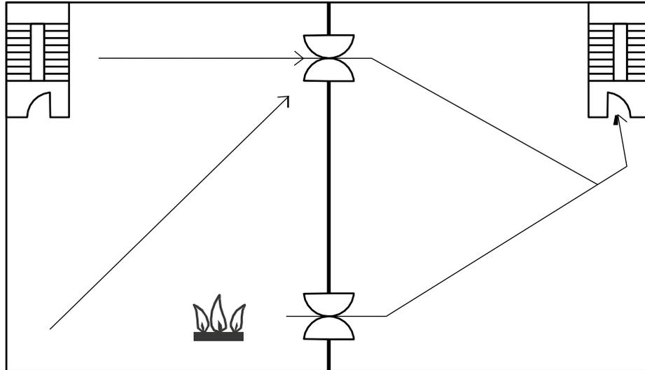
Storey divided into two refuges by compartment wall (stairways not provided with wheelchair space).
