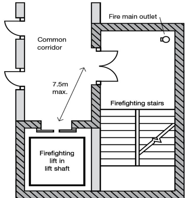
□ Minimum fire resistance 60 minutes from both sides with 30 minute fire doors
