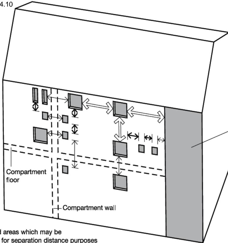
The unprotected area of the external wall of a stairway forming a protected shaft may be disregarded for separation distance purposes
