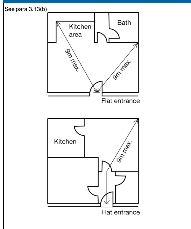
**3.14** Where any flat has an alternative exit and the habitable rooms do not have direct access to the entrance hall (see Diagram 4):
