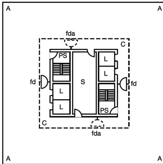
**Note:** The doors at both ends of the area marked 'S' should be self-closing fire doors unless the area is sub-divided such that any fire in that area will not be able to prejudice both sections of corridor at the same time. If that area is a lift lobby, doors should be provided as shown in Figure 8 in BS 5588: Part 11: 1997.
