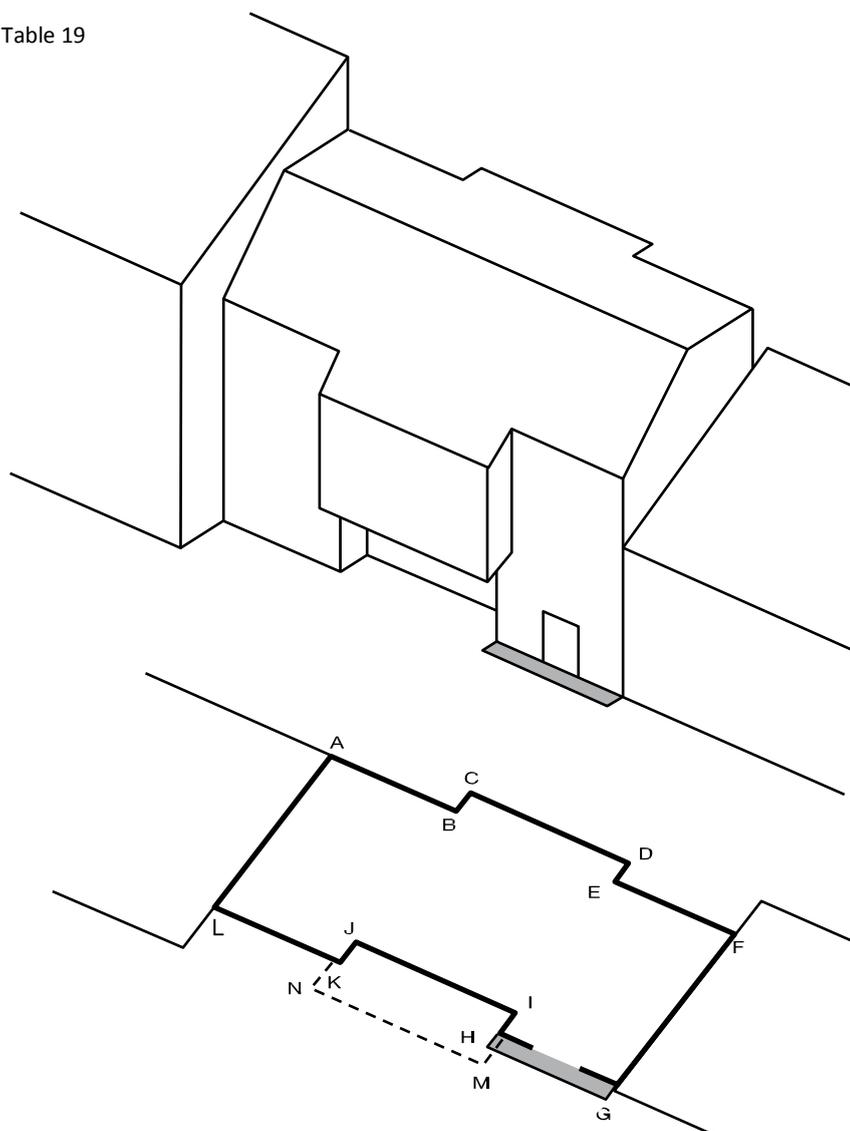
Plan of building AFGL where AL and FG are walls in common with other buildings.
