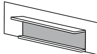
Projections from the building line such as a canopy or a loading platform can be ignored when assessing separation distance. This would not apply to an enclosed loading bay, for example if the illustration had shown side walls beneath the canopy.
